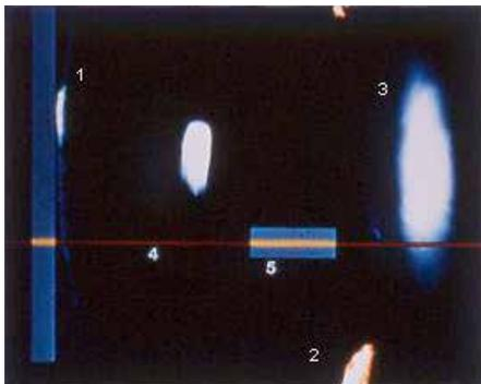
The instrument measures back-scattered light from small molecules such as proteins and this is called laser flare photometry. The measurement units of back scattered light from small molecules are number of photons per milliseconds (ph/ms). The amount of back-scattered light is proportional to the concentration and size of proteins in the aqueous humor and is so indicating the level of inflammation.
